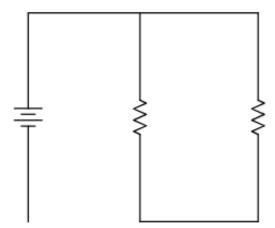
The figure shows a battery connected to two resistors. Is there current in the resistors? What evidence or reasoning supports the claim?
