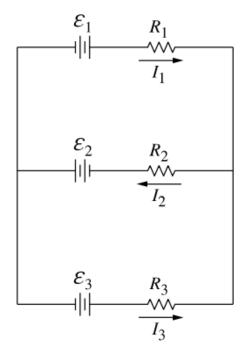
The figure shows a circuit with three batteries and three resistors with the emf of each battery and the resistance of each resistor as indicated. Write an equation that expresses a Kirchoff's loop rule for a portion of the circuit.
