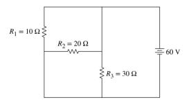
The figure shows three resistors connected to a battery, with the resistances and emf indicated. Rank the potential differences  $\Delta V_1$ ,  $\Delta V_2$ , and  $\Delta V_3$  across resistors  $R_1$ ,  $R_2$ , and  $R_3$ , respectively?
