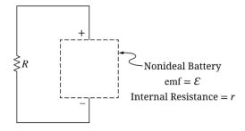
The figure shows a circuit with resistor of resistance R connected to a nonideal battery. The battery has emf  $\epsilon$  and an internal resistance r. What is the current generated by the battery?
