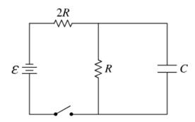
In the circuit shown in the figure, the switch has initially been opened for a long time. The switch is then closed. Immediately after the switch is closed, the current in resistor 2R is  $I_i$ . A long time after the switch is closed, the current in the resistor 2R is  $I_f$ . What is the approximate value of the ratio  $\frac{I_f}{I_f}$ ?
