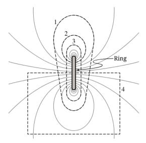
A circular ring carries and electric current. The magnetic field diagram shown is in a plane that passes through the center of the ring, and which is perpendicular to the plane of the ring. Four parths 1, 2, 3, and 4, represented by dashed lines, are in the plane of the magnetic field along which the integral  $\oint \vec{B} \cdot d\vec{l}$  may be evaluated. Which of the paths would yield a result of zero when evaluating this integral?
