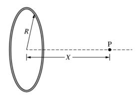
A circular loop of wire has a radius R and carries a current I. Point P is along the central axis of the loop a distance X away from the center of the loop, as shown. What is the magnitude of the magnetic field at point P?
