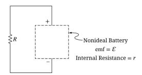
The figure shows a circuit with resistor of resistance R connected to a nonideal battery. The battery has emf  $\epsilon$  and an internal resistance r. What is the current generated by the battery?
