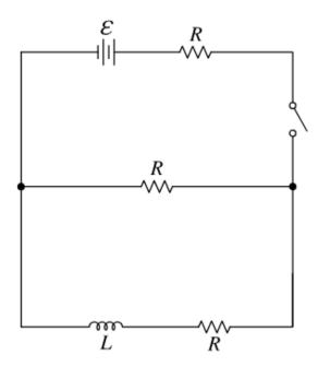
A circuit is constructed from a battery of emf  $\epsilon$ , a switch, an inductor of inductance L, and three identical resistors of resistance R, connected as shown in the diagram. The switch is initially open. Write an expression that best indicates the energy stored in the inductor a long time after the switch has been closed.
