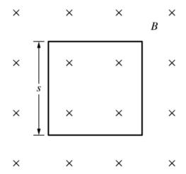
A single loop of wire with resistance R is placed in a magnetic field that is directed into the page, as shown. The loop is a square with each side having a length s. The magnitude of the magnetic field as a function of time is given by  $B(t)=4t^3+3$ . What is the magnitude of the current induced in the wire due to the changing magnetic field as a function of time.
