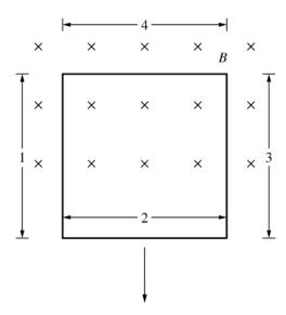
A square loop os wire is moving at speed v as it exists a magnetic field directed into the page, as shown. Segments 1 and 3 of the wire are halfway in the magnetic field, Segment 2 has completely exited the magnetic field, and Segment 4 is completely in the magnetic field. Which segment(s) of the loop, if any, will experience a magnetic force from the external magnetic field?
