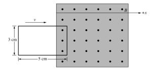
A 3.0 cm wide and 5.0 cm long rectangular loop of conducting wire of resistance  $0.2\Omega$ , is moved at a constant speed of 3.0 m/s to the right. The loop enters, passes through, and exits a 0.5 T magnetic field directed out of the page, as shown. The loop is always moved at a constant speed. What is the work done by the magnetic field on the loop?
