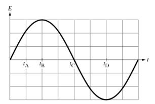
A circuit is constructed by connecting a capacitor and an inductor. The electric field E in the capacitor varies sinusoidally with time t. Times  $t_A, t_B, t_C$ , and  $t_D$  are indicated in the figure. Rank the magnitudes of the currents  $I_A, I_B, I_C$  and  $I_D$  in the inductor at times  $t_A, t_B, t_C$ , and  $t_D$  respectively.
