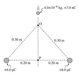
A small sphere of mass  $4.0\times10^{-6}$  kg and net charge +3.0 nC is moving along a straight line that is equidistant from two larger fixed spheres, as shown in the figure. Each fixed sphere has a net charge of  $+6.0\mu$ C. The moving sphere first passes through point O, which is 0.30 m from each fixed sphere, and later point P, which is 0.20 m from each fixed sphere.
