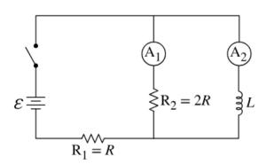
A circuit containing an inductor of inductance L, resistors  $R_1$  and  $R_2$  of resistance R and 2R, respectively, a battery of emf  $\epsilon$ , two ammeters, and a switch is constructed as shown in the diagram. After the switch is closed and the circuit reaches steady state, how does the current  $I_1$  measured by Ammeter  $A_1$  compare to the current  $I_2$  measured by Ammeter  $A_2$ , and why?
