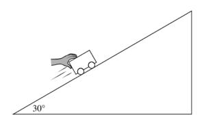
A  $0.250~\rm kg$  cart is being pushed up a track that is inclined at  $30^\circ$  above the horizontal as shown. Friction between the cart and the track is negligible. Calculate the minimum power required to push the cart up the track at a constant speed of  $2.4~\rm m/s$ .
