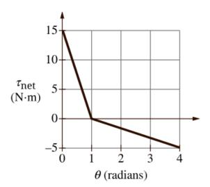
An object can rotate about an axis passing through its center of mass. At t=0, the object is spinning in the positive direction and has an initial angular position of zero. The graph represents the net torque  $\tau_{net}$  exerted on the object as a function of angular position  $\theta$ . What is the total work done on the object and the maximum rotational kinetic energy of the object as it rotates from 0 radians to 4 radians?
