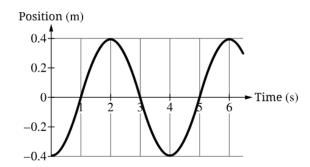
The graph shows the position x as a function of time t for an object in one-dimensional simple harmonic motion. Write an expression that gives the object's velocity as a function of t.
