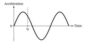
An object undergoes simple harmonic motion. The graph shows the acceleration of the object as a function of time, and at time  $t_0$  the acceleration is in the positive direction as indicated. Describe the object's displacement and velocity at time  $t_0$ .
